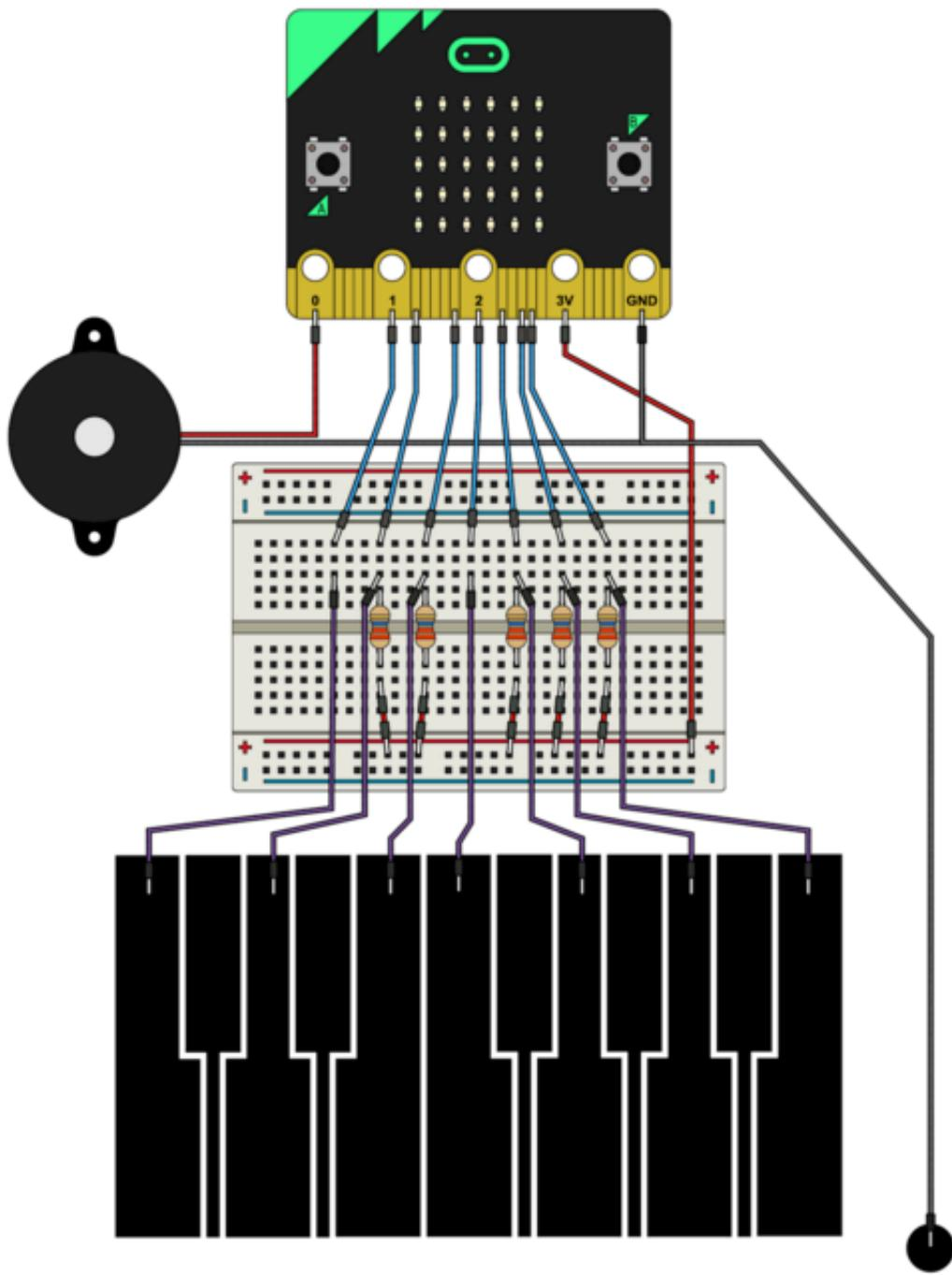
Because we need more than three pins for this project, we need to use the other pins on the edge connector, using the breakout board.
