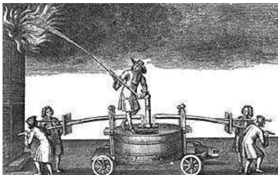
A C17th 'fire engine' showing the see-saw action of the pump
