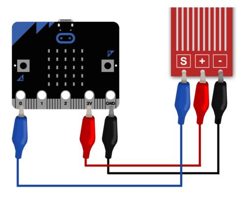
Using the crocodile clips and wires, connect the negative (-) pin on the sensor to GND on the BBC micro:bit, the positive (+) pin on the sensor to 3V and the signal (s) pin to Pin 0, 1 or 2. Here, we've used Pin 0.
